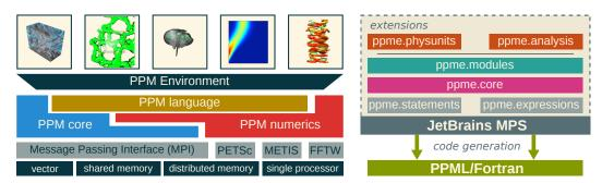
Fig. 10. PPME: New access layer to the underlying PPML.
