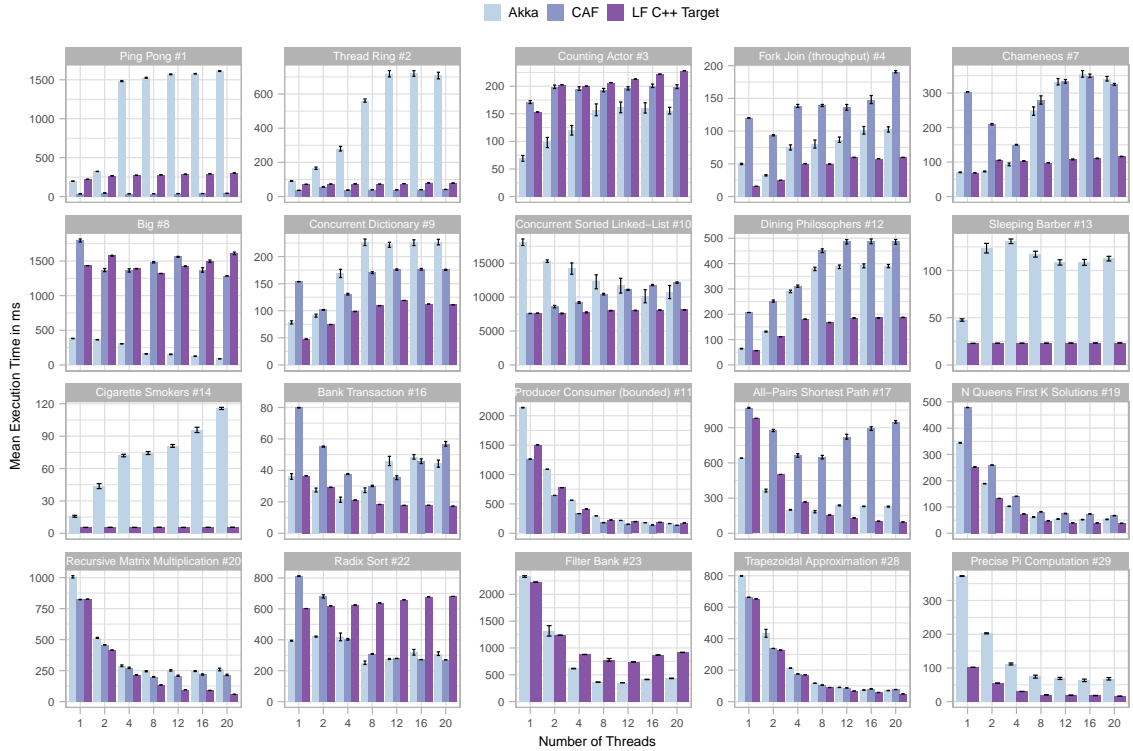
Fig. 14. Mean execution times and 99% confidence intervals for various Savina benchmarks implemented in LF, CAF, and Akka, measured for a varying number of worker threads. The numbers prefixed with # are benchmark IDs as listed in [41].
