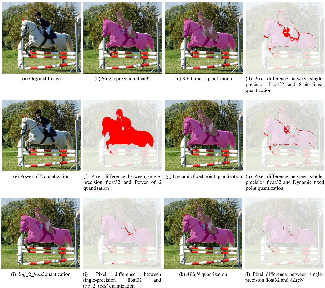
FIGURE 18. Object detection comparison with different quantization schemes using FCN8 [26] network on PASCAL VOC 2012 validation set [27].
