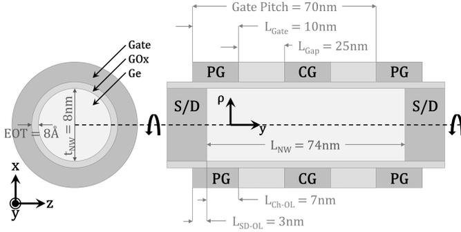
**Fig. 2:** Simulated nanowire structure for TCAD model including the dimensions compliant to a  $14\text{nm}$  technology node.
