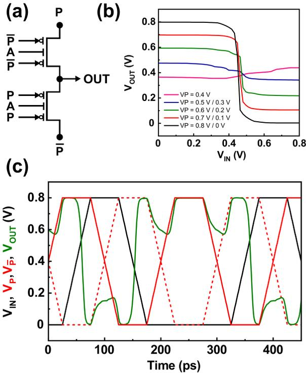
**Fig. 5:** Dynamically reconfigurable inverter (a) circuit diagram with applied signals (b) dynamic voltage transfer curve (VTC) and (c) transient behavior during the reconfiguration process.
