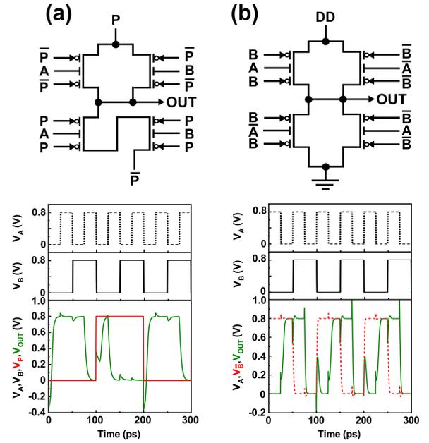
**Fig. 6:** Base versions of two reconfigurable circuits and their simulated transient behavior. (a) Dynamically reconfigurable NAND/NOR with dedicated program signal, (b) static 2-XOR exploiting internal reconfiguration.
