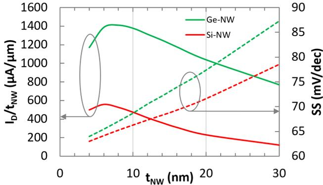
**Fig. 3:** Drain current normalized to the nanowire diameter as well as subthreshold swing as functions of the nanowire diameter of a simulated Ge-NW-RFET (green) as well as Si-NW-RFET (red).  $V_D = 0.8\text{ V}$ ,  $V_{PG} = 0.8\text{ V}$  and  $V_{CG} = 0.8\text{ V}$
