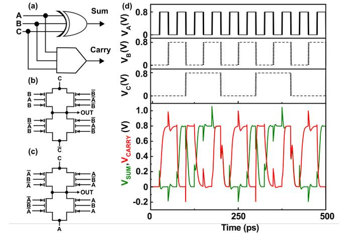
**Fig. 7:** 1-bit Full adder as proposed in [51]. (a) Generic 1bFA design with separated paths for SUM and Carry function comprise of (b) 3-XOR and (c) 3-MAJ. (d) Transient output sequence for the 1bFA.
