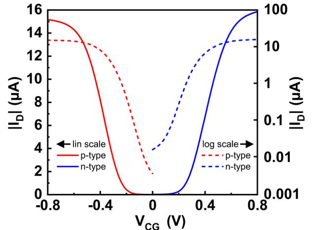
**Fig. 1:** Simulated transfer characteristics in linear (full lines) and logarithmic (dashed lines) scale of a single Ge-NW-RFET structure related to the 14 nm TCAD model for n-type (blue,  $V_D = 0.8$  V,  $V_{PG} = 0.8$  V) as well as p-type (red,  $V_D = -0.8$  V,  $V_{PG} = -0.8$  V) configuration.
