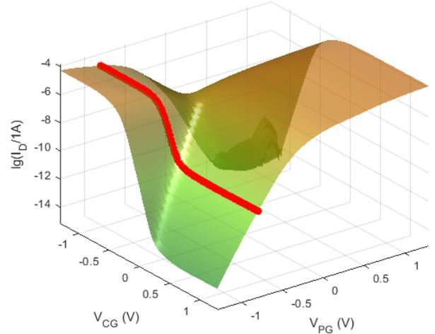
**Fig. 4:** TCAD simulation of a drain current field in logarithmic scale at  $V_D = -0.8\text{ V}$ . The red line shows the transfer characteristic for  $V_{PG} = -0.8\text{ V}$ .
