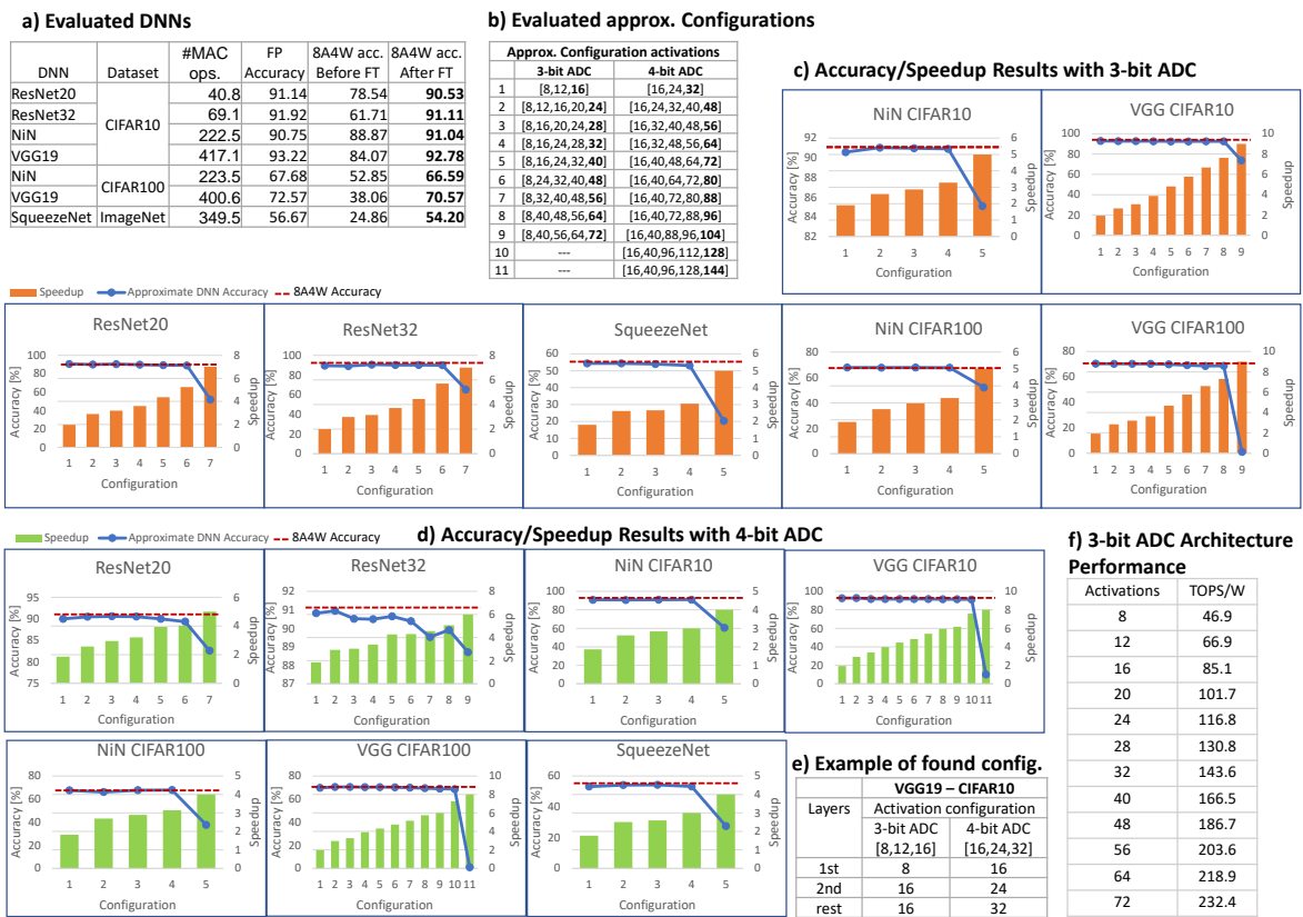
Figure 4: a) Evaluated DNNs num. of parameters, MAC ops and accuracies at Floating point(FP) representation as well as at 8A4W before and after fine-tuning (FT). b) All evaluated approximate configurations for 3-bit and 4-bit ADCs. c) 3-bit ADC solutions with best accuracy/speedup trade-off for each configuration in b) that maintains the 8A4W DNN accuracy. d) 4-bit ADC solutions with best accuracy/speedup trade-off for each configuration in b) that maintains the 8A4W DNN accuracy. e) Example of found configurations for model VGG19 for CIFAR10 (3-bit and 4-bit architecture, 1st set of possible configurations): 1st and 2nd layers require more accuracy, rest of layers can be computed with max. approximation level. f) Performance of 3-bit ADC in-memory accelerator from [12] with each possible activation configuration.
