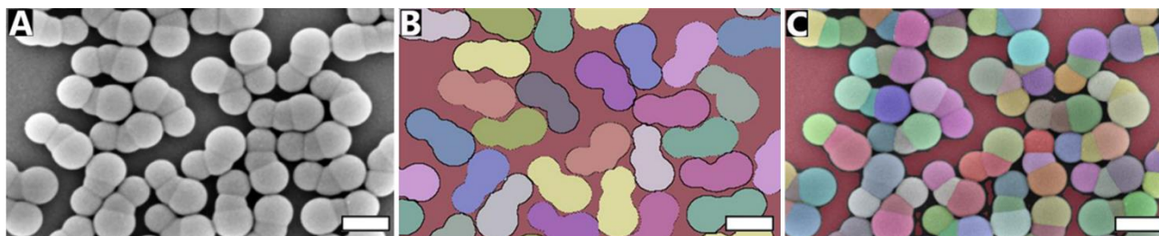
Figure 1. Scanning electron micrograph of colloidal trimers (A). Two image segmentation processes are performed: (B) identification of the trimers as a whole (B), and then their segments (C). The two datasets can be combined through mathematical processing, thereby providing additional information. The scale bars are 250 nm.
